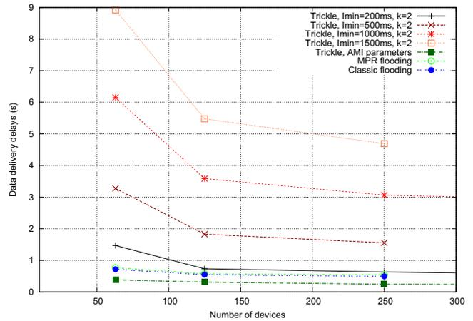
Figure 4. Variable Density: Data Delivery Delays.
